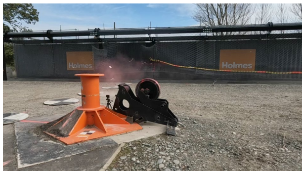
Figure 23 Full-scale testing, snapback system successfully redirecting parted mooring line - Keane, R (2024)
