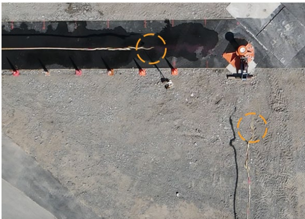
Figure 5 85t, 72mm, mixed PP/PE mooring line failed at 51% LDBF (D/d 5:1); each end travelling at 150 km/h, representing failure towards both vessel and shore sides - HSLP, (2025)
