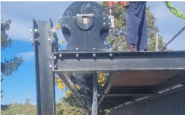
Figure 9 Snapback protection roller system being retracted to demonstrate rapid operation - Keane R, (2024)
