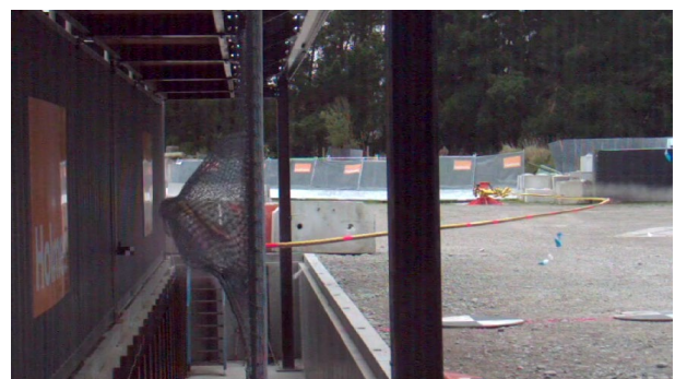
Figure 22 Deflection of arresting structure observed during testing – Keane R, (2024)
