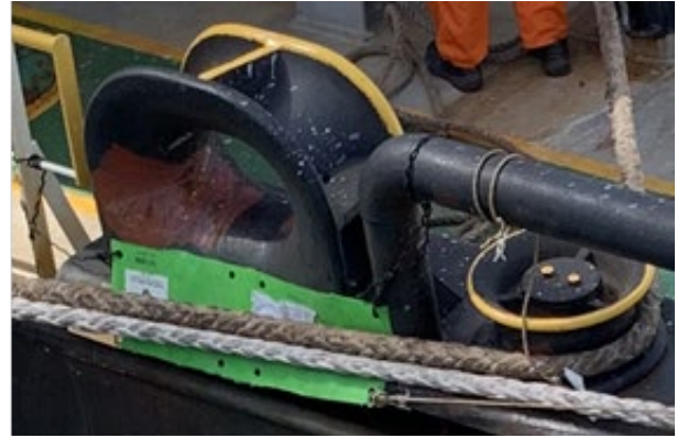
Figure 6 Typical fairleads on dry bulk vessel which could be classed as sub optimal when discussing D/d ratio - BMA, (2021)
