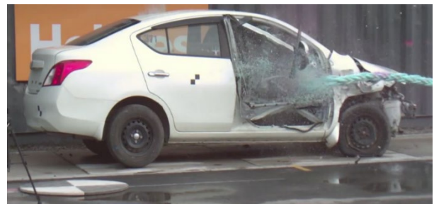
Figure 2 Severity of snapback illustrated: vehicle door struck by line at ~770 km/h, causing catastrophic damage - HSLP, (2025).
