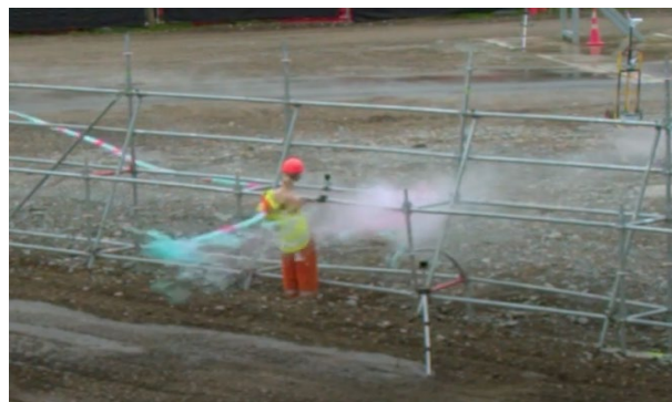
Figure 2: A temporary arresting structure developed using conventional methods, unsuccessfully arresting ruptured line - Smith A.S, (2021).
