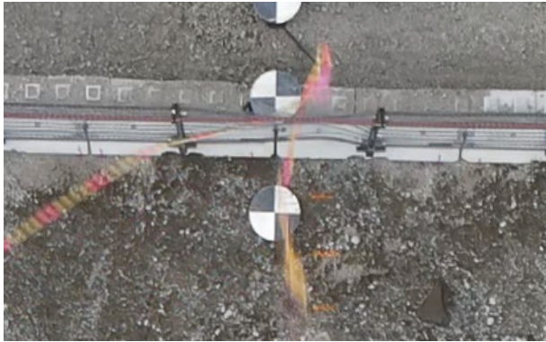
Figure 9: Geobrug F1 Debris Fence during Research + Development snapback test to establish baseline, unsuccessfully arresting ruptured mooring line - Smith A.S, (2021).
