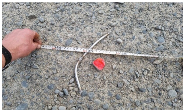
Figure 4: Debris 5 recovered during snapback testing of a non-proprietary rigid arresting structure - Keane R, (2024).
