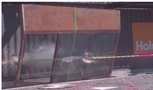
Figure 1: A snapback event penetrating a conventionally designed operator cabin with multilayered toughened glass during base line testing - Keane R, (2024).
